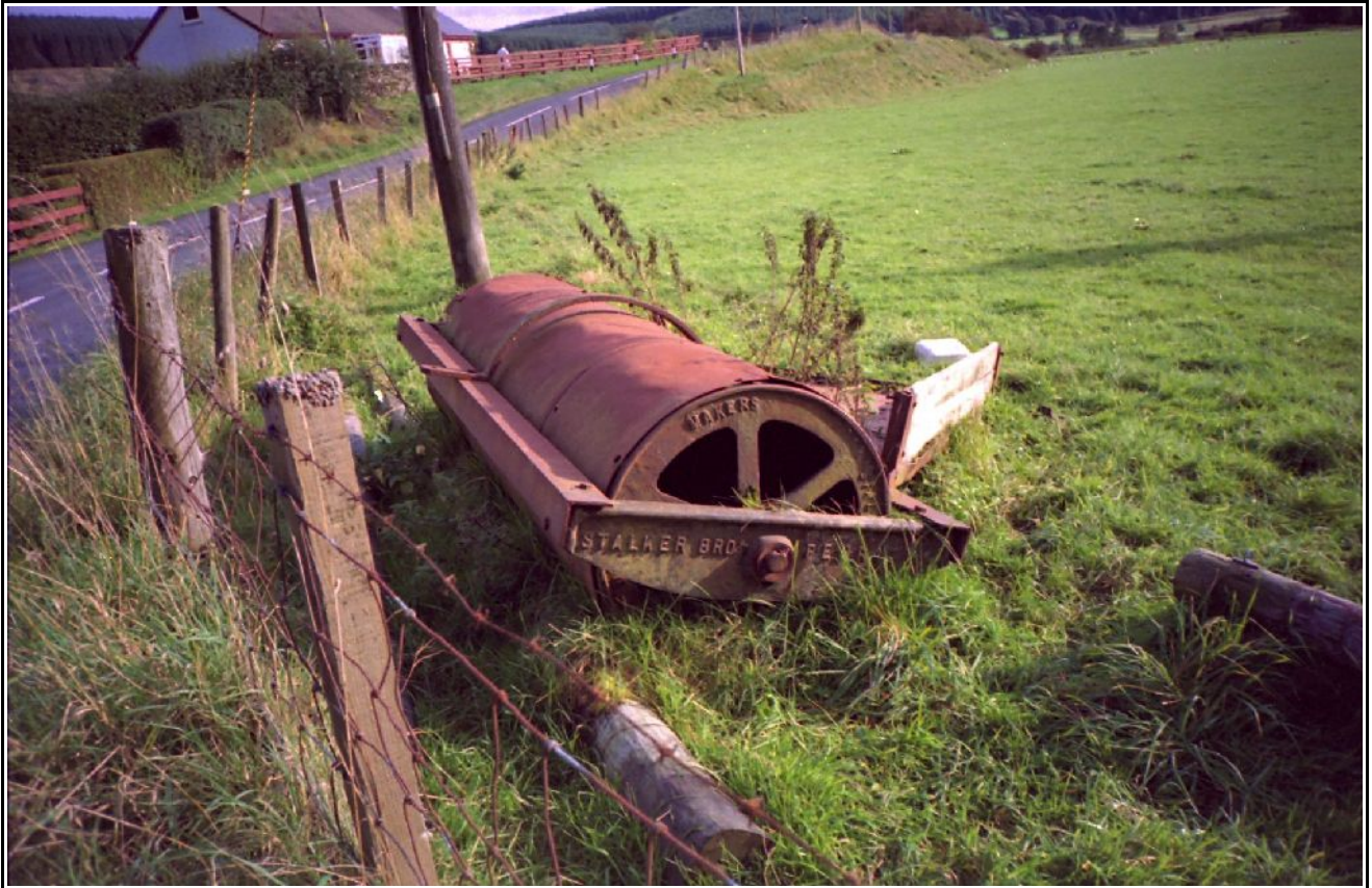
Stalker Brothers, Penrith, Cumberland - built cast-iron meadow roller, that I discovered lying in marshy ground at the side of a country lane near Westerhill, Dumfriesshire.
