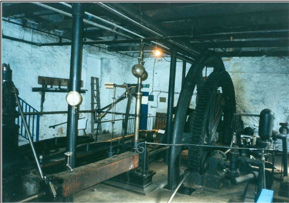
Horizontal steam engine at Keithbank Mill, Blairgowrie, Perthshire, thought to have been constructed by Carmichael of Dundee in 1864.
