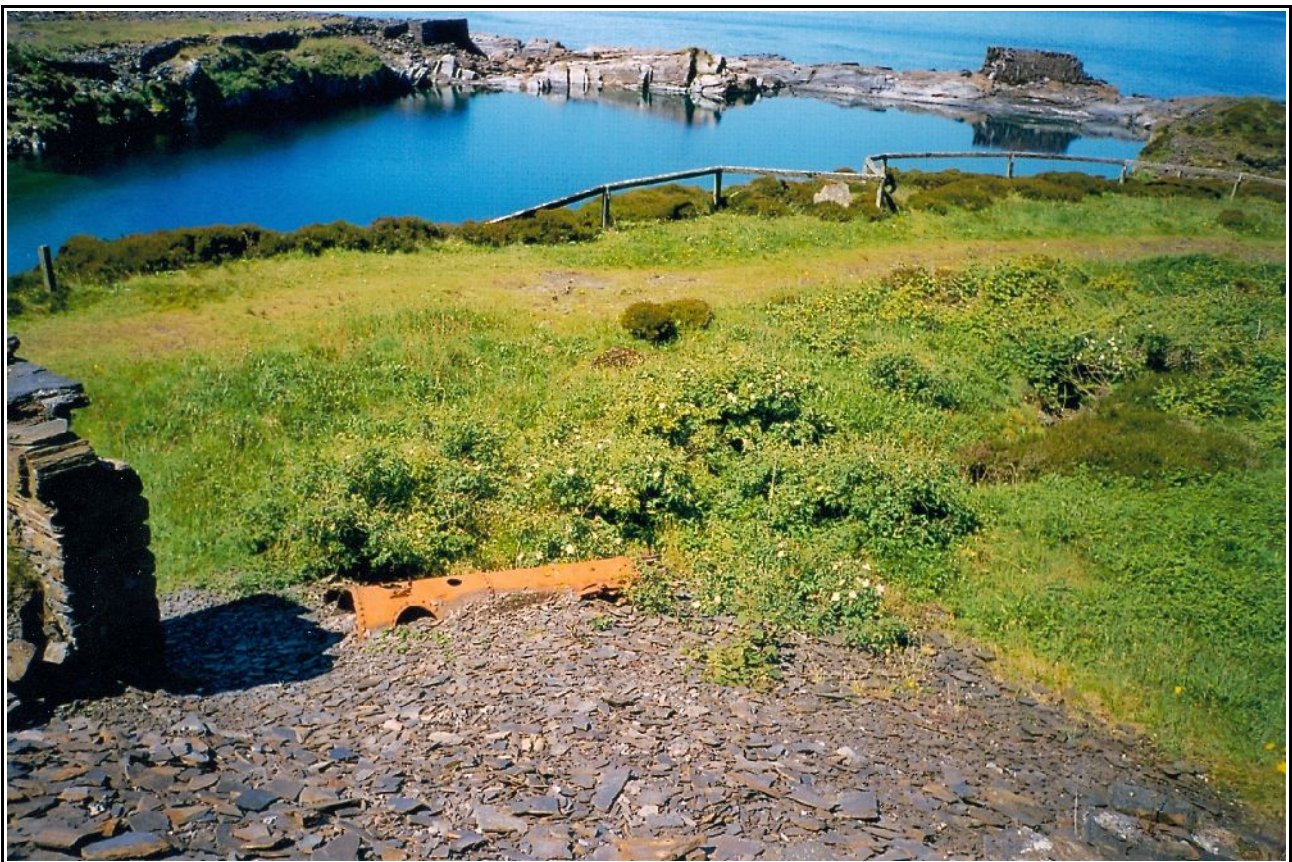
An old vertical cross-tube steam boiler almost buried in slate waste. It was possibly used originally to power a steam crane in the slate quarry.
