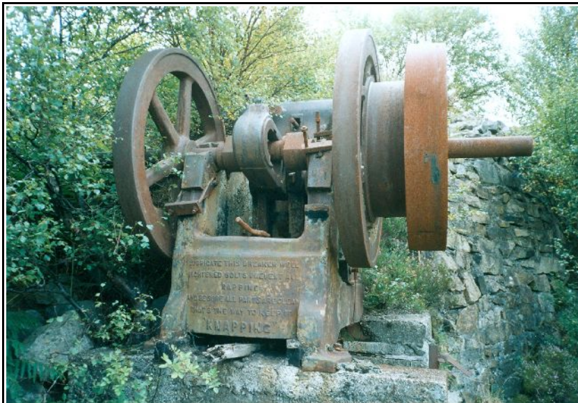
At a long-abandoned quarry at Luib, Isle of Skye, stands this interesting belt-driven rock crusher.
